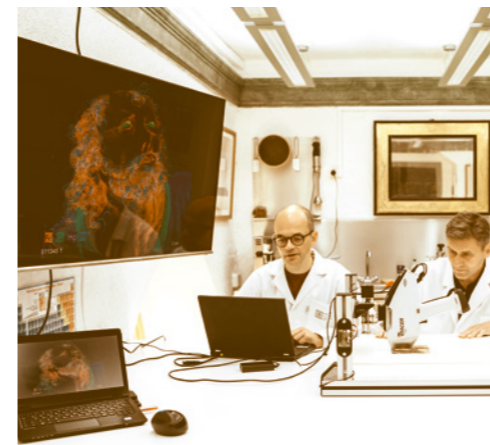
Researchers investigate a Cranach drawing using X-ray fluorescence analysis
