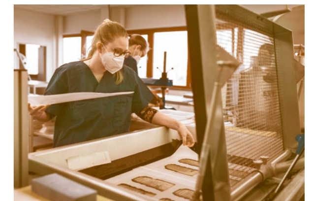
Reconstruction of fragmented double-leaf sheets in the leaf-casting machine
